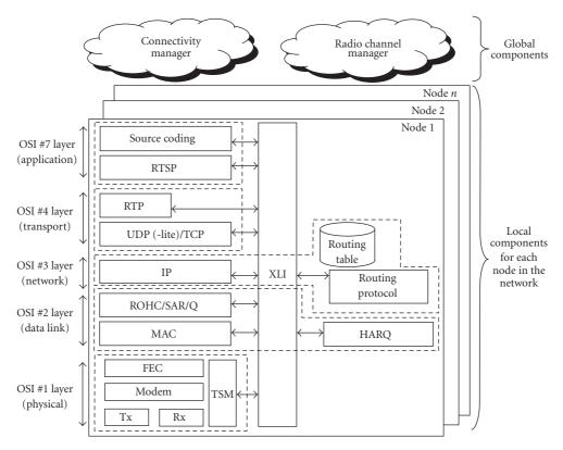
FIGURE 1: Overall protocol architecture.
