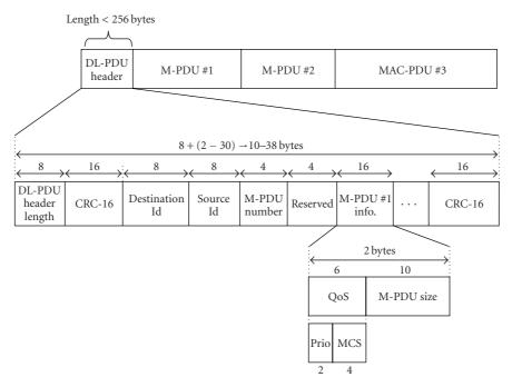
FIGURE 3: Bit-oriented implementation: example of UDP/IP framing.
