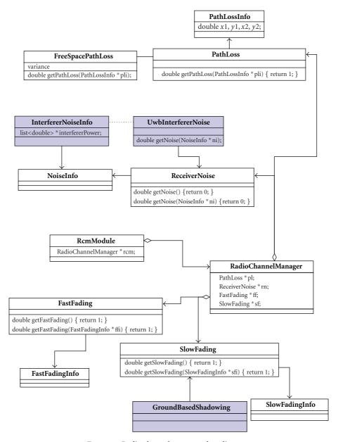
FIGURE 5: Radio channel manager class diagram.
