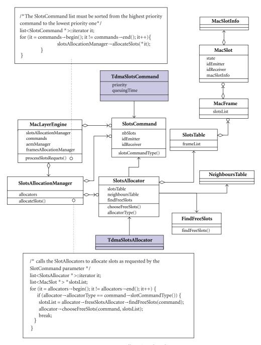
FIGURE 4: Resource allocation class diagram.
