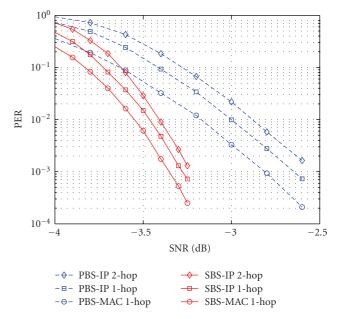
FIGURE 8: PBS and SBS performance comparison with IR-HARQ, for  $N=3,\,P=8,$  and C=24.
