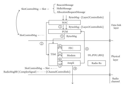
FIGURE 6: Radio access sequence diagram at transmission side.
