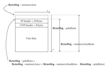
FIGURE 2: Example of Application Programming Interface: transmitting real bits.
