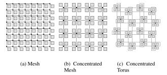
Figure 2. Mesh, concentrated mesh, and concentrated torus topology. The concentrated topologies require a larger-radix switch, but reduce the average hop count.
