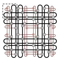
Figure 3. The photonic torus topology, studied in [15]. Switch blocks are abbreviated: X -  $4 \times 4$  nonblocking, I - injection, E - ejection, G - gateway. Zoomed in view of the dotted box is shown in Figure 4.
